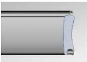
**Aluminium lath** with optimized profile section, winding and guide properties, resulting in low-noise and low abrasion running. Plastic side locks help prevent lateral displacement of the lath, also aiding the smooth-running operation. Manufacture dimensions max. 5,000 x 5,000 mm. TH80 ECO Speed max. 5,000 x 8,000 mm. End profile natural aluminium (untreated) as standard.
