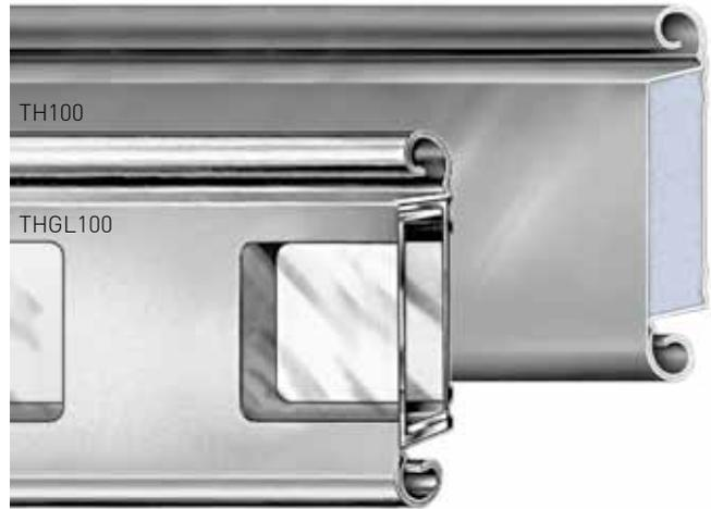
**100mm, double skinned**, aluminium lath. A more conventional profile section, approximately 23mm thick. With thermal-insulating polyurethane, non-plasticized foam core with adhesive-free connection with the shell, thus providing a high level of surface stability.
