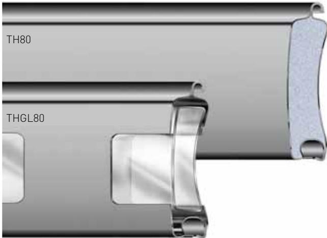
**80mm, double skinned**, aluminium lath, approximately 20mm thick. With thermal-insulating polyurethane, non-plasticized foam core with adhesive-free connection to the shell, thus providing the highest level of surface stability. The especially developed profile section formed in high-quality optics, enables significantly tighter winding of the door curtain, allowing lower headroom requirements.
