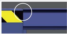
Flush joint between main deck and lip when fully extended
